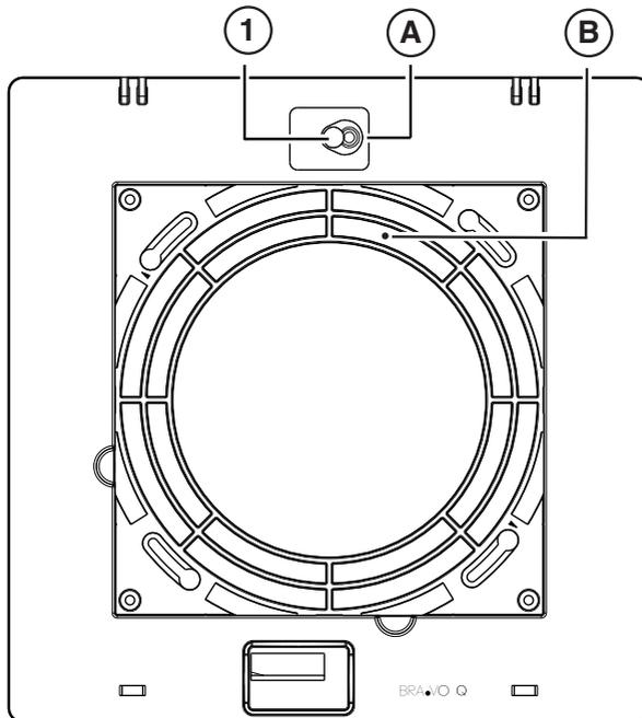
**(A)** = This button activates pairing, or rather product coupling with the household Wi-Fi. Press and hold (indicatively for 5 sec.) until the blue LED **(1)** starts flashing. Then release the button.
